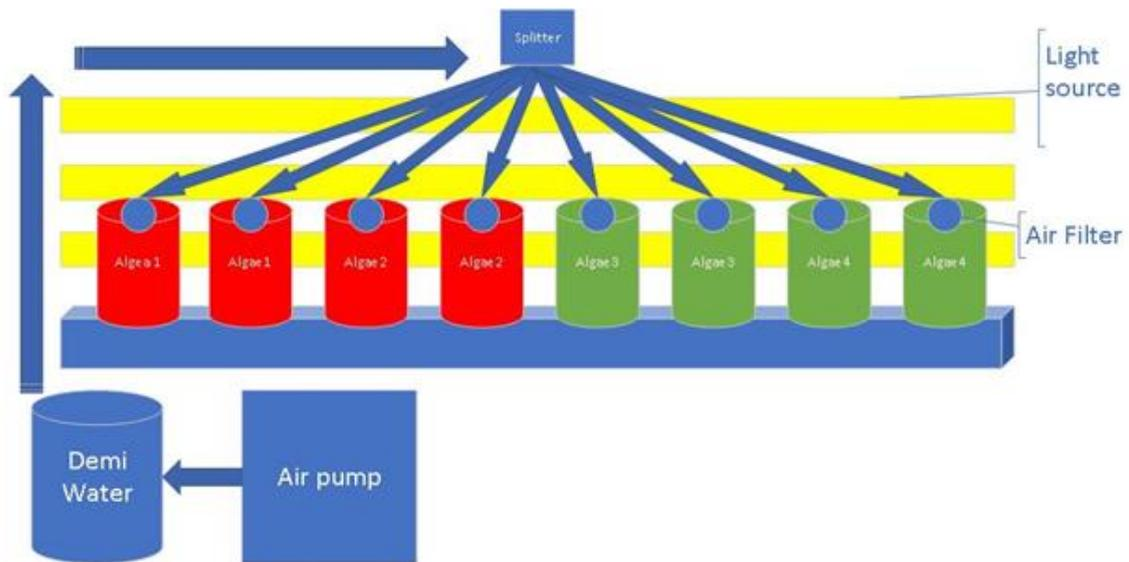
Figure 3: a schematic overview of the culture setup using 8 different bottles
