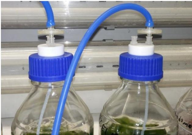
*Figure 2: culture vessel with air filter and input / output cap*
