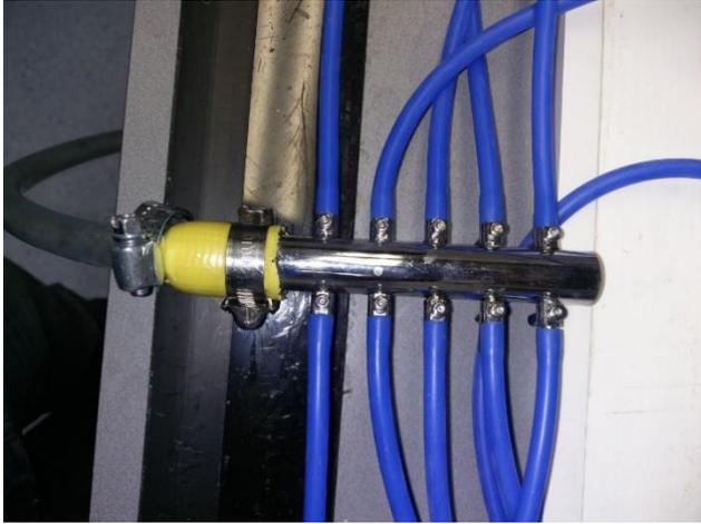
*Figure 1: air being split to different culture vessels*
